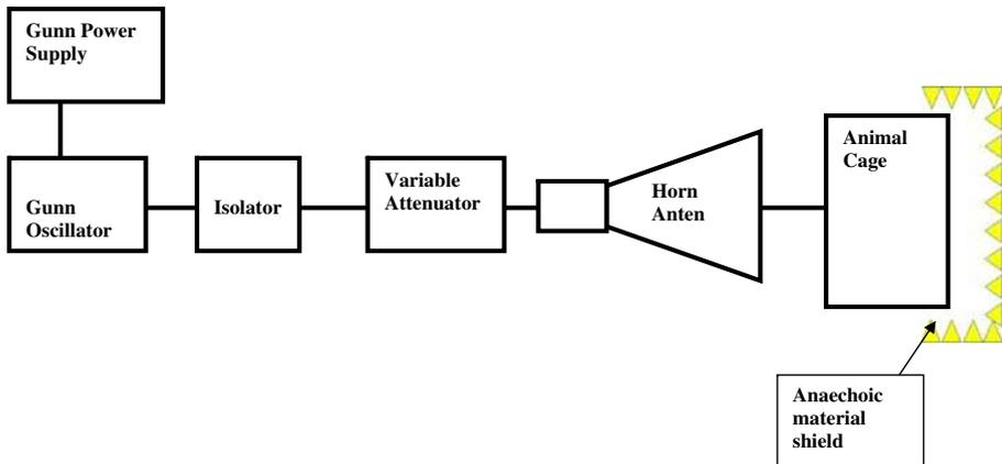
**Fig. 1** Schematic diagram of 50-GHz radiation source
